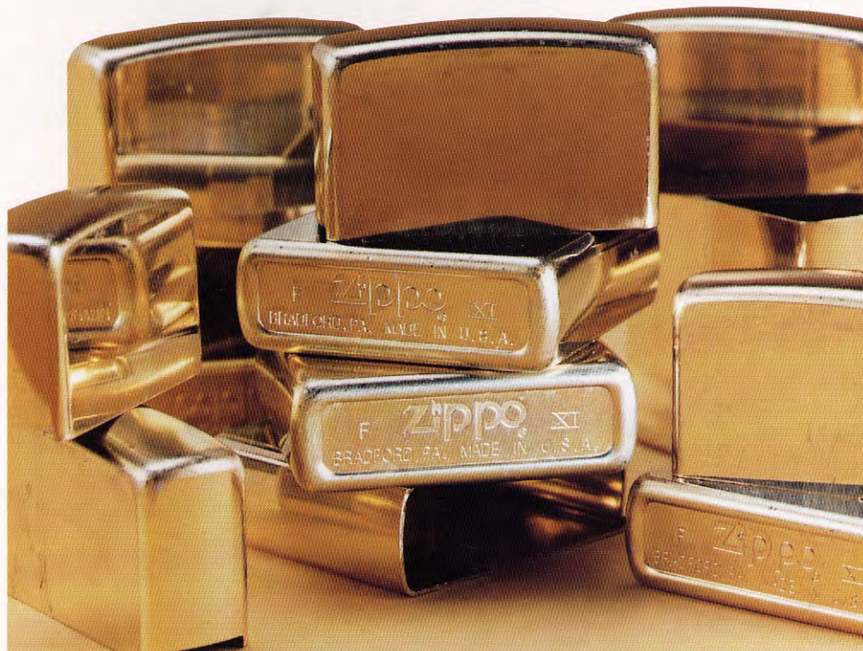
Minster presses stamp the top and bottom casings for Zippo lighters.
