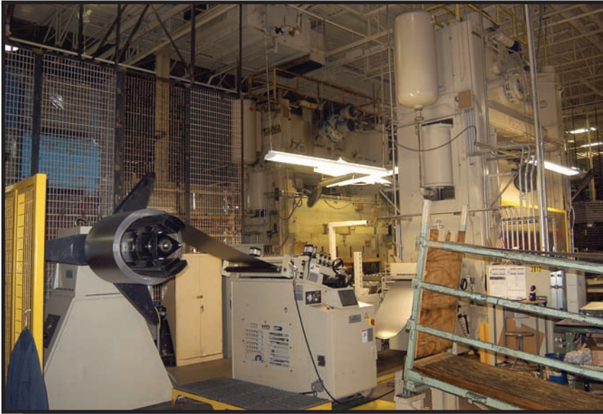
Retrofit Minster feed line on a 600-ton Verson press at Whirlpool Corporation's Findlay, Ohio manufacturing facility.
