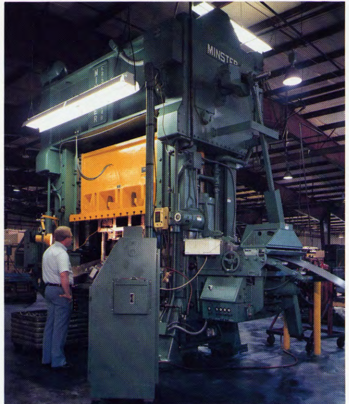
A new E2-200 with Minster double roll rack and pinion feed produces clutch pedals from .210" thick material at 65 SPM.
