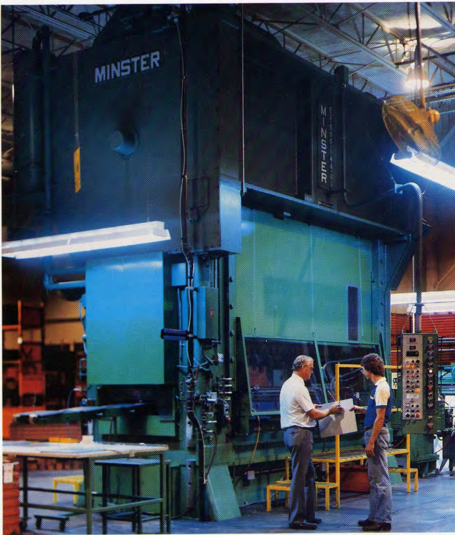
This new E2-500-144 is the largest automatic, coil fed press ever installed at Steelcase.
