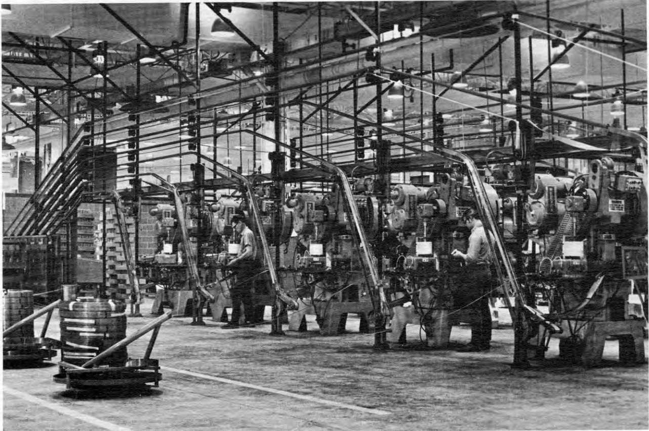
Ten B1 presses in unusual automated line at Signode Corporation.
