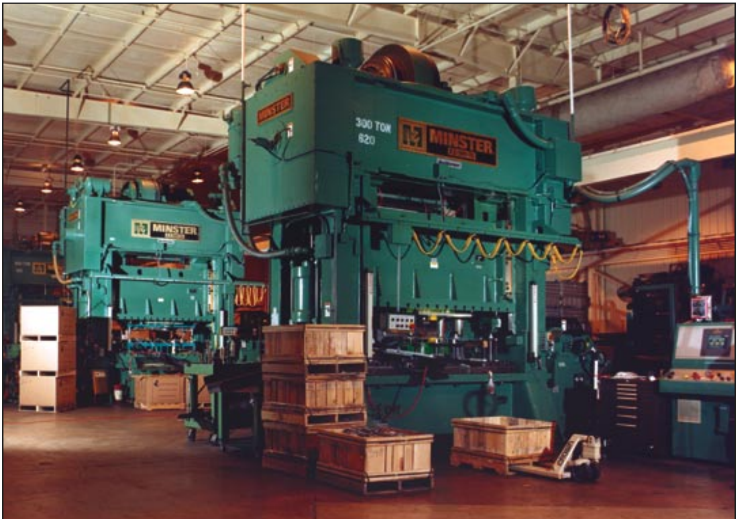
E2-300 ton presses are used for many of the in-die assembly applications at Rockford Toolcraft.
