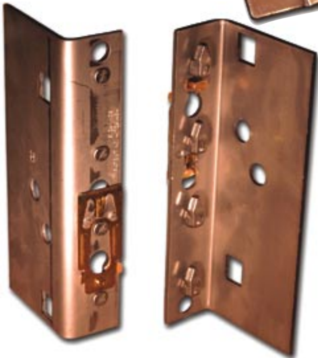
Heavy gauge shelving bracket parts produced on a two-out die. Each bracket is staked with L-studs and a safety clip.
