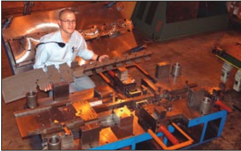
Press Dept. Foreman Seth Doolan shows a die and stock strip from Rockford Toolcraft.
