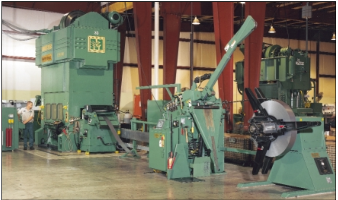
This Minster E2H-350 press includes a completely integrated coil line featuring a Minster Feed, Straightener and Reel.
