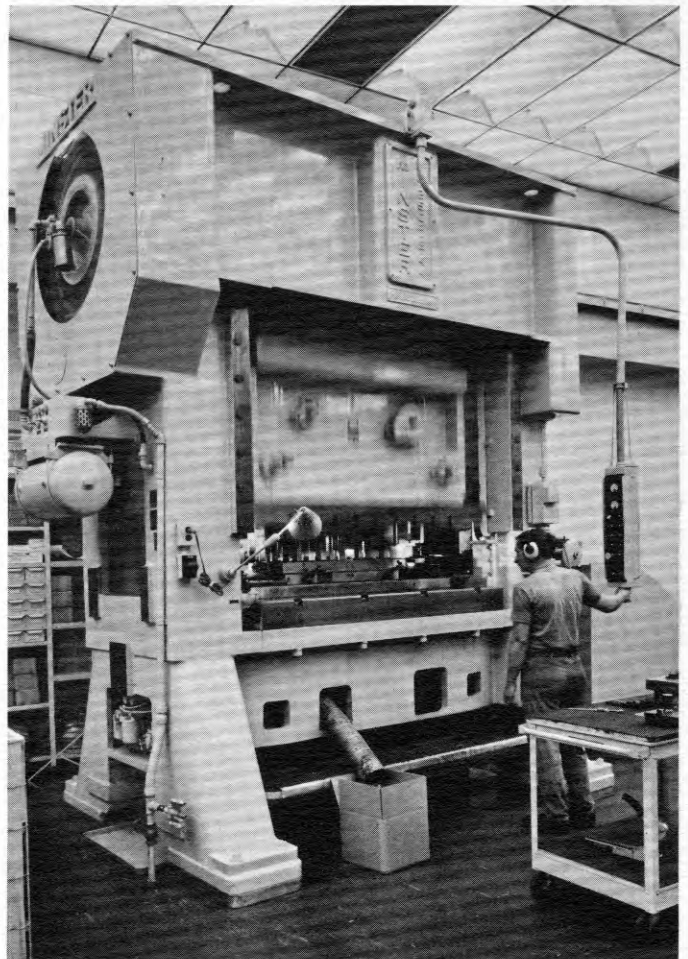
Production run in progress in Oberg's Minster E2-250 try-out and production press.
