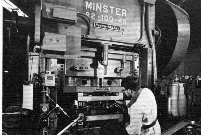
P2-100 press is used to cold-form fuse part at 40 to 50 spm in one operation using rotary die.
