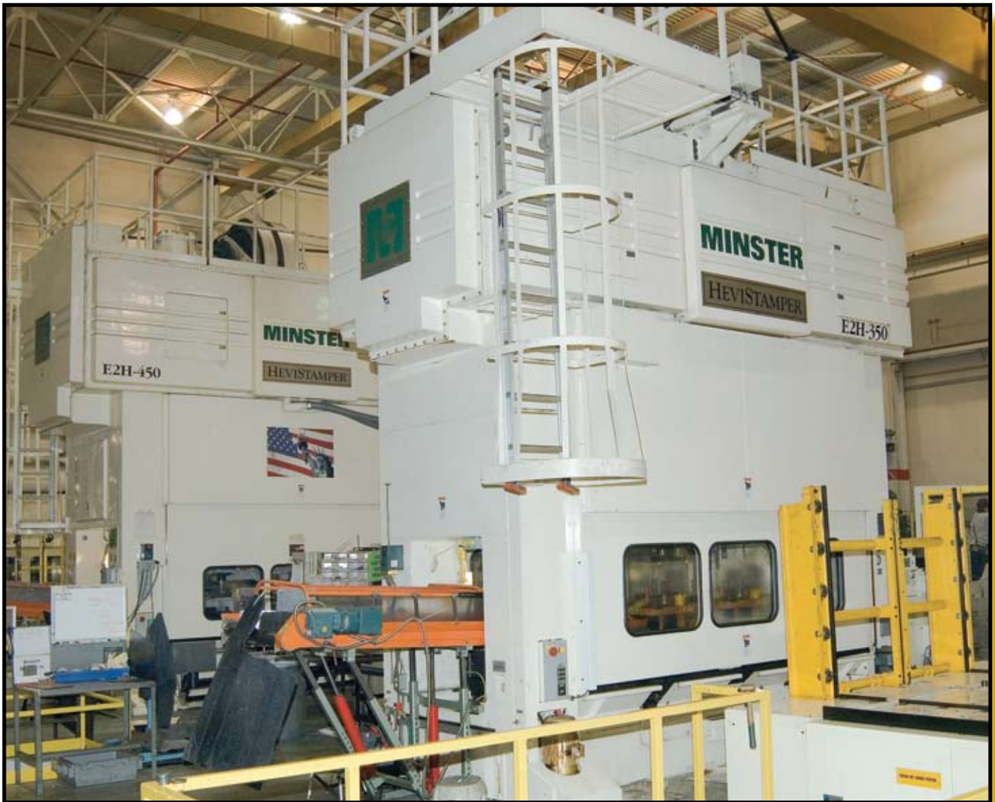
E2H presses help with the stamping of high tensile automotive frame components at Kalida Manufacturing, Inc.
