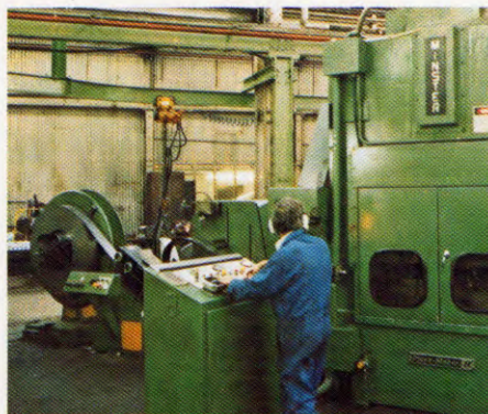
The Minster "S-Loop" Coil Handling System and Cam Feed keeps material flowing through this press.
