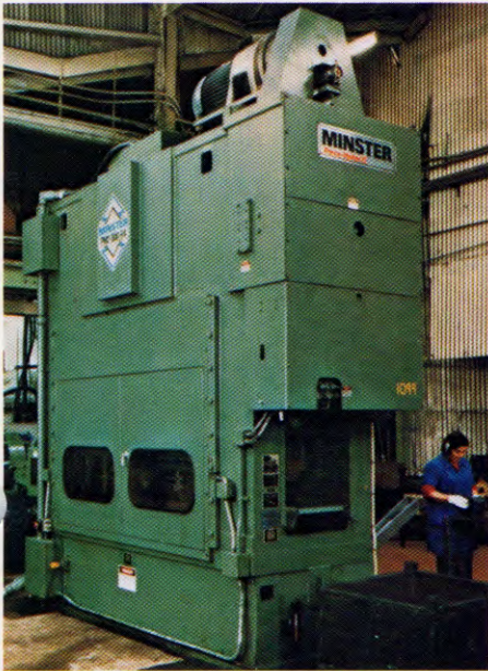
Dynamically balanced 300 ton Minster dominates the press line at Scott's Cheshire facility.
