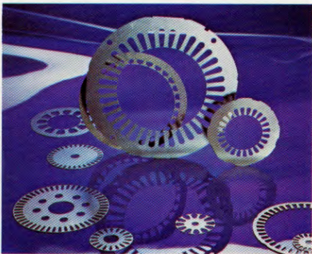
Rotor and stator laminations at the Geo. L. Scott Company are used in the manufacture of A.C. and D.C. motors — powering everything from home appliances to express trains.
