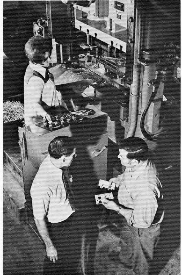
Ed Reitter, Press Room Foreman, on right, and Glenn Mesler, Plant Manager at Collier Steel Corporation discuss high speed production of garage door hinges on Minster P2-150 press.
