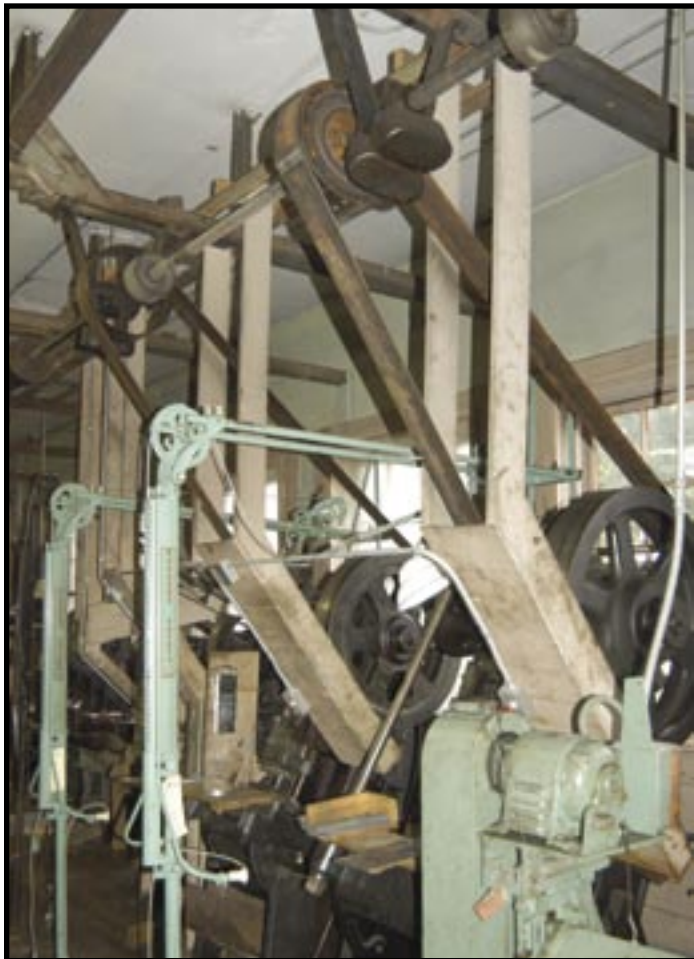
A ceiling-mounted line shaft provides the power for many of the machine tools at the Bluffton Slaw Cutter Company, which produces a variety of vegetable and fruit choppers, graters and slicers.
