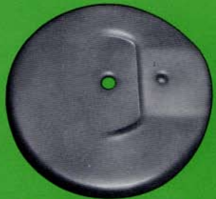
Shells blanked, drawn and formed on compound dies from ¾" thick steel coil.
