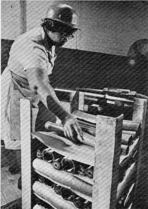
Strings of laminations weighing as much as 40 lbs. each are carefully stacked in heavy duty containers.
