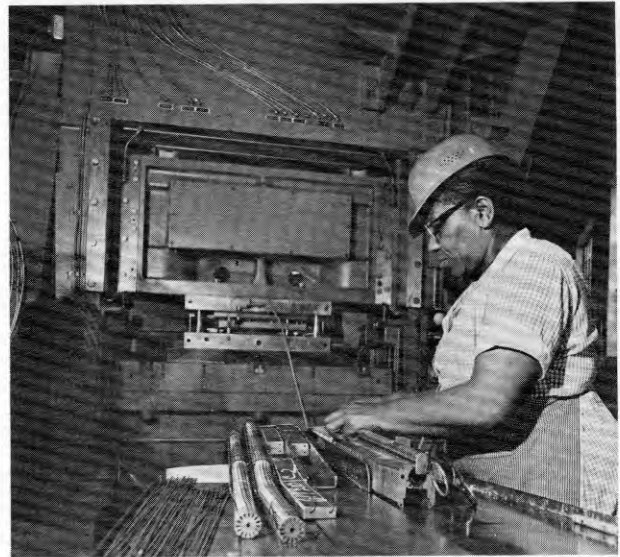
Two full sets of laminations for shaded pole induction motors are made with a two-up die on each cycle of this Minster press. Each set consists of rotor, stator and bar laminations.
